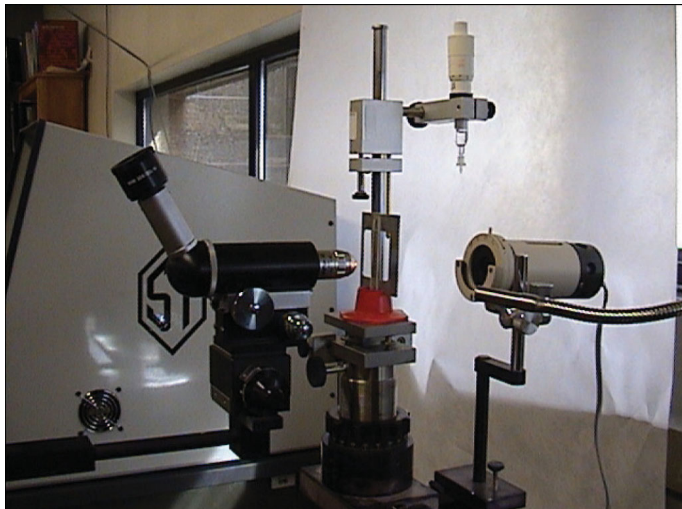
Figure 3 A hollow fiber goniometer developed by combining an NRL Rame–Hart model 100 contact angle goniometer with a Rame–Hart, model 104 wetometer.
